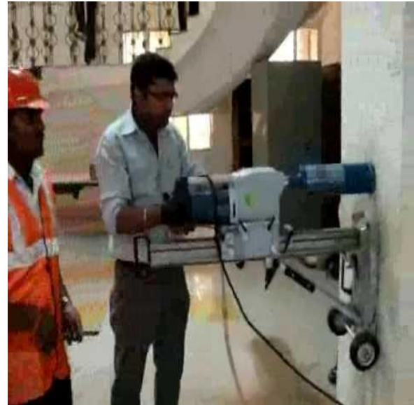
Fig 2.12: Core test equipment and sample extrusion of core
