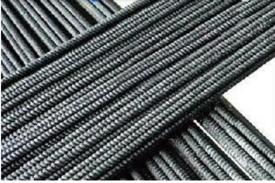
Fig 3.7: Carbon fibre reinforcement
