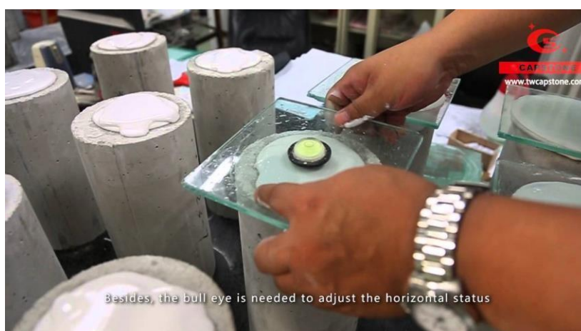
Fig 2.13: Capping of concrete Core
